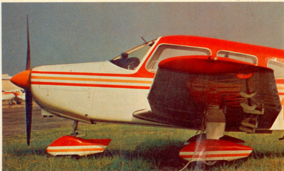
The new airplane's wing is tapered, swept and drooped.
