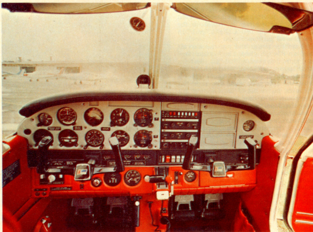
The panel of N55151 includes optional Narco radios and a gyro instrument package.
